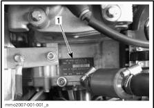
V800 ENGINE TYPE 1. Engine serial number
