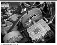
TYPICAL Step 1: Slip the belt over the top edge of the sliding half Step 2: Turn driven pulley at the same time
