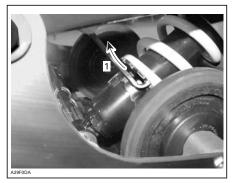
1. Use adjuster wrench provided in tool kit to increase preload
