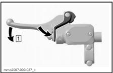
TYPICAL — RELEASE MECHANISM Step 1: Squeeze brake lever
