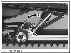
TYPICAL Step 1: Pull on handle Step 2: Turn to increase spring preload
