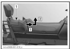
**TYPICAL** Step 1: Slide seat forward Step 2: Lift seat to remove
