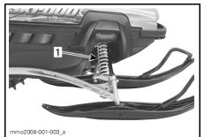
TYPICAL — FRONT SUSPENSION 1. Front shock — handling
