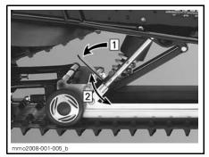
**TYPICAL** Step 1: Pull on handle Step 2: Turn to decrease spring preload
