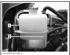
SKANDIC SWT V800 — EXPANSION RESERVOIR NEAR MUFFLER 1. Maximum
