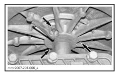
**NOTE:** Allen screws must be restrained while tightening lock nut to prevent throwing adjustment out.
