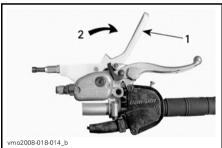
ON POSITION 1. Parking brake lever 2. Pull to apply parking brake
