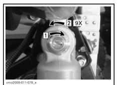
FACTORY SETTING Step 1: Turn clockwise until it stops Step 2: Turn counterclockwise (9 clicks)
