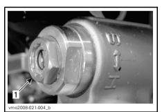
TYPICAL — DS 450 X ONLY 1. High speed compression adjuster (17 mm wrench)
