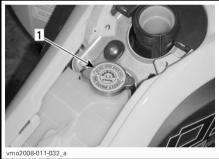
UNDERNEATH ACCESS COVER 1. Coolant tank cap
