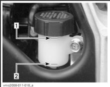
RH SIDE OF VEHICLE 1. Maximum level (MAX) 2. Minimum level (MIN)
