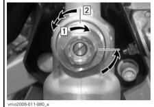
DS 450 X — FACTORY SETTING Step 1: Turn clockwise until it stops Step 2: Turn counterclockwise (3/4 of a turn)
