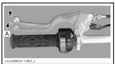
CLUTCH LEVER — PROPER ADJUSTMENT A. 10 to 15 mm
