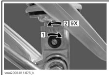
FACTORY SETTING Step 1: Turn clockwise until it stops Step 2: Turn counterclockwise (9 clicks)
