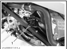
LH SIDE OF VEHICLE 1. Oil tank dipstick
