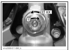
DS 450 X — FACTORY SETTING Step 1: Turn clockwise until it stops Step 2: Turn counterclockwise (8 clicks)
