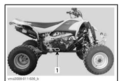
TYPICAI — ENGINE SERIAI NUMBER IARFI 1. E.I.N. (Engine Identification Number)
