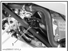
1. Engine oil tank cap
