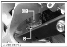
PRELOAD ADJUSTMENT Step 1: Loosen top locking ring Step 2: Turn adjusting ring accordingly Step 3: Tighten top locking ring
