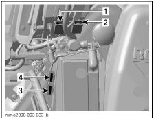
RH SIDE OF ENGINE COMPARTMENT 1. 15 A headlight fuse (RED/ORANGE wire) 2. 20 A accessories fuse (RED/YELLOW wire)
