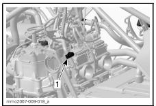
TYPICAL — REMOVE BELT GUARD 1. Carburetor valve
