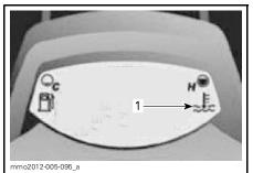
OPTIONAL MODULE INSTALLED 1. Overheating indicator
