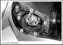
Step 1: Push both sides Step 2: Pull to release 1. Retaining clip
