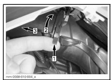
TYPICAL Step 1: Lift tab Step 2: Twist adapter Step 3: Pull off
