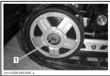
1. RH rear idler wheel retaining screw
