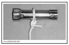
Attach the other end of emergency rope to the starter clip supplied in the tool kit.
