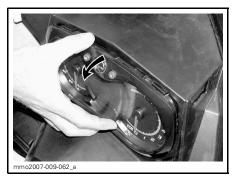
3. Disconnect burnt bulb connector. Remove the rubber boot.
