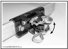
HITCH MOVES FREELY WHEN TOWING
