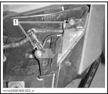
1. Taillight housing retaining screws
