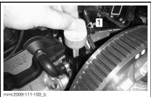
LH SIDE OF VEHICLE 1. Oil tank dipstick
