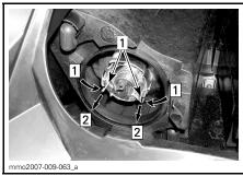
Step 1: Push both sides Step 2: Pull to release 1. Retaining clip
