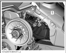
LH SIDE OF VEHICLE 1. Oil tank dipstick
