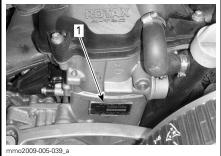
1200 4-TEC ENGINE 1. Engine identification number
