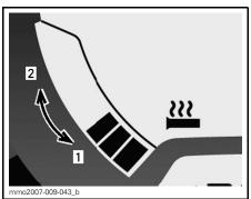
HEATING INTENSITY DISPLAY 1. Less heat 2. More heat
