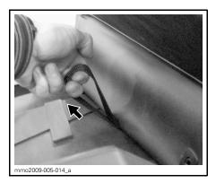
3. Lift up the rear end of seat and gently pull back just enough to expose the accessories connector.
