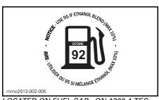
LOCATED ON FUEL CAP - ON 1200 4-TEC AND 900 ACE ENGINES (IN COUNTRIES USING RON OCTANE RATINGS)
