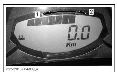
HEATING INTENSITY DISPLAY 1. Less heat 2. More heat
