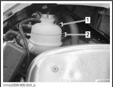
1200 4-TEC MODEL SHOWN 1. Coolant tank 2. COLD LEVEL line
