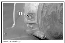
TYPICAL - 600 HO E-TEC AND 800R E-TEC 1. Magnetic check plug
