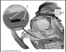
**PIVOT THE ACCESS COVER** 1. Retaining screws
