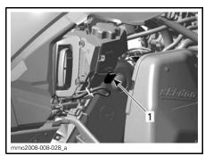
TYPICAL - RH SIDE OF ENGINE COMPARTMENT 1. 5 A start/RER fuse
