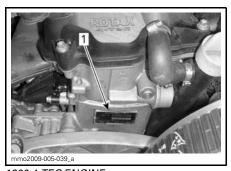
**1200 4-TEC ENGINE**1. Engine identification number
