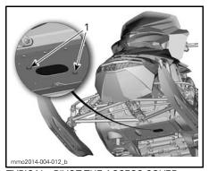
TYPICAL - PIVOT THE ACCESS COVER 1. Retaining screws
