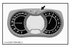
To change HOURS, while the value of HOURS is blinking, use the SET (S) button to change hours.
