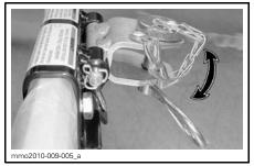
HITCH MOVES FREELY WHEN TOWING
