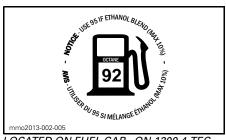
LOCATED ON FUEL CAP - ON 1200 4-TEC AND ACE ENGINES - IN COUNTRIES USING RON OCTANE RATINGS
