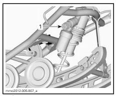
Center shock compression damping adjustment knob
