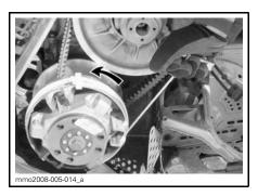
Pull the rope using a sharp, crisp pull so the rope comes free of the drive pulley. Start engine as per usual manual starting.
