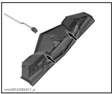
RETAINING BOLTS SECURING TAILLIGHT TO TAILLIGHT SUPPORT
