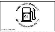
LOCATED ON FUEL CAP - ON 600 HO E-TEC ENGINE (IN COUNTRIES USING PUMP POSTED AKI (RON+MON)/2 OCTANE RATINGS)
