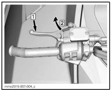
TYPICAL — ENGAGE MECHANISM Step 1: Apply and hold brake Step 2: Lock brake lever using parking brake lever
