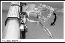
HITCH MOVES FREELY WHEN TOWING
