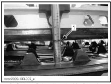
1. Deflection O-ring aligned with slider shoe
