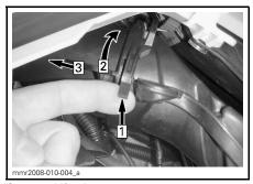
Step 1: Lift tab Step 2: Twist tube Step 3: Pull forward
