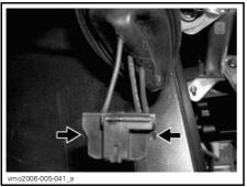
PUSH ON LOCKING TAB TO UNLOCK CONNECTOR
