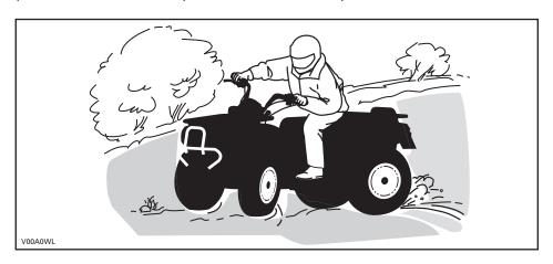
If you do get into a slide or skid, it may help to turn the handlebar into the direction of the skid until you regain control. Never jam the brakes and lock the wheels.
