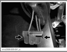
PUSH ON LOCKING TAB TO UNLOCK CONNECTOR
