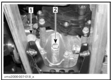
1. Oil level plug 2. Oil drain plug
