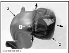
CVT AIR INLET REMOVED FOR CLARITY PURPOSE
