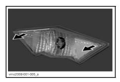
Turn and pull light socket to expose bulb
