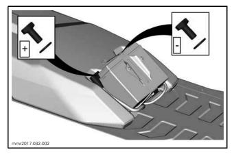
4. Remove battery hold down bracket.
