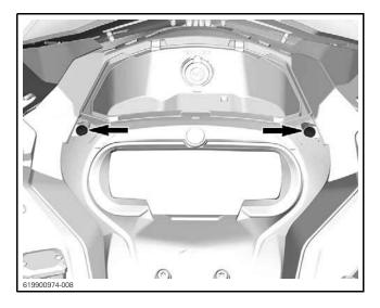
4. Lift the front of the gauge support, then slide it forward to remove it.
