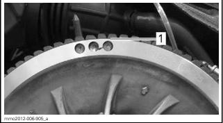
TYPICAL - PRELIMINARY SETTING 1. Lowest portion of cogs even with driven pulley edge
