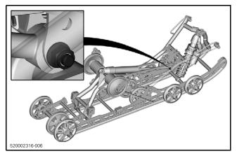
**NOTE:** It may be necessary to lower the vehicle and slightly compress the suspension to remove the load.
