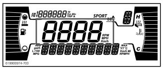
Display the RPM of the engine or the vehicle speed in Km/h or MPH.
