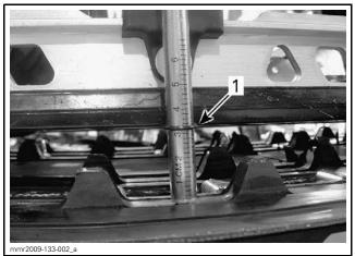
1. Deflection O-ring aligned with slider shoe
