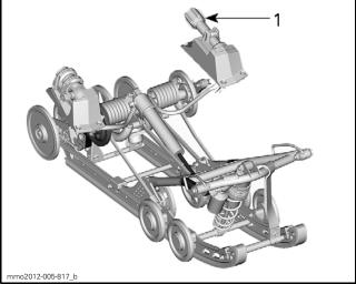
rMOTION WITH QUICK ADJUST 1. LH side knob to adjust spring preload
