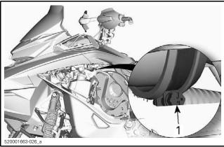
8. Loosen the air intake duct clamp.
