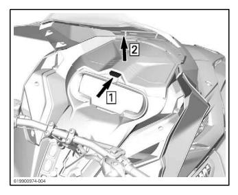
3. Remove the gauge support retaining screws.
