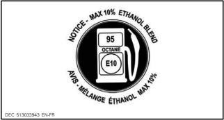
ON FUEL CAP - ON 600R E-TEC AND 850 E-TEC ENGINE IN COUNTRIES USING RON OCTANE RATINGS
