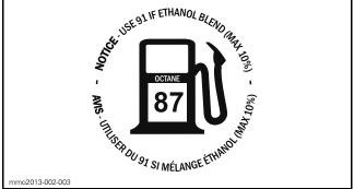
LOCATED ON FUEL CAP - ON 600 EFI ENGINE (IN COUNTRIES USING PUMP POSTED AKI (RON+MON)/2 OCTANE RATINGS)
