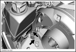
Step 1: Slide toward engine Step 2: Slide toward front of vehicle
