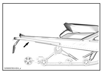
5. Pull on the oil pump cable - at the adjustment - until the exhaust gas turns to darker smoke.
