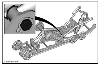
6. Remove the cam, pivot 180°, reinstall in the rail.
