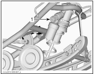
1. Center shock compression damping adjustment knob
