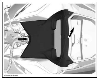
5. Disconnect the gauge and remove from vehicle.
