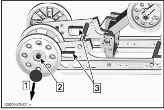
Step 1: Remove cap Step 2: Loosen the axle screw or nut Step 3: Tighten or loosen adjustment screws
