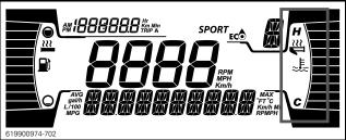
HEATED THROTTLE LEVER DISPLAY
