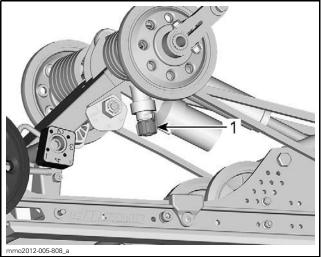
**TYPICAL** - **rMOTION WITHOUT QUICK ADJUST** 1. Compression damping adjustment button
