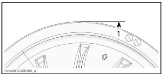
600 EFI - PRELIMINARY SETTING 1. Drive belt outer surface is even with the driven pulley edge
