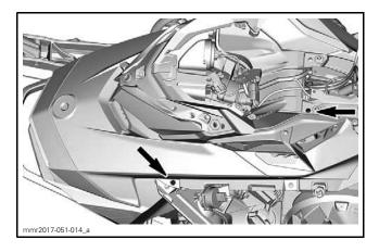
10. Free the rear end hooks of the upper body module from the slots in the console.
