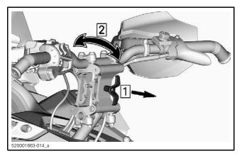
Move the handlebar back and forth to make sure mechanism is securely engaged.
