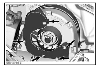
Secure in place by sliding it behind the tabs.
