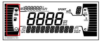
Heated grips will be in OFF position when there are no bars displayed on the gauge.
