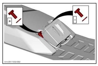
4. Remove battery hold down bracket.
