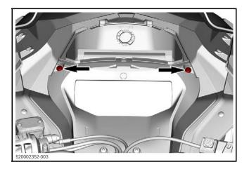
4. Lift the front of the gauge support , then slide it forward to remove it.
