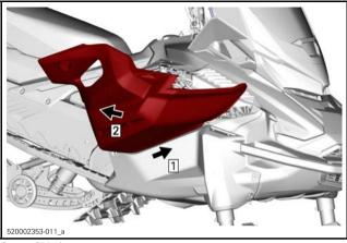
Step 1: Slide front Step 2: Pull out from side bottom pan
