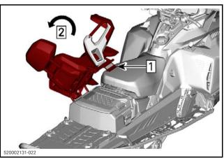
Step 1: Unlock seat latch Step 2: Tilt passenger seat
