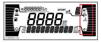
Heated throttle lever will be in OFF position when there are no bars displayed on the gauge.
