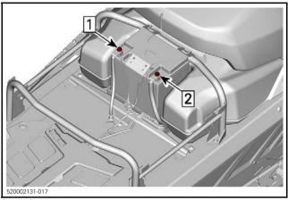
Step 1: Disconnect negative Step 2: Disconnect positive
