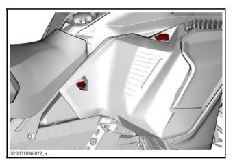
When closing panel, make sure latches are locked securely.
