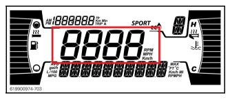
Display the RPM of engine or vehicle speed in Km/h or MPH.
