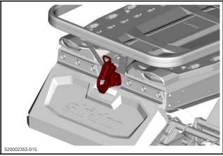
To open the hook, push and turn the handle to retract locking plate.
