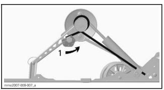
TYPICAL — RH SIDE 1. Adjust spring preload
