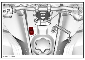
To activate Standard mode when in Sport mode, press bottom end of switch once.
