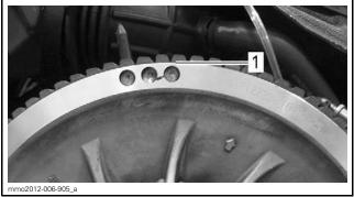
600R E-TEC - PRELIMINARY SETTING 1. Lowest portion of cogs even with the driven pulley edge
