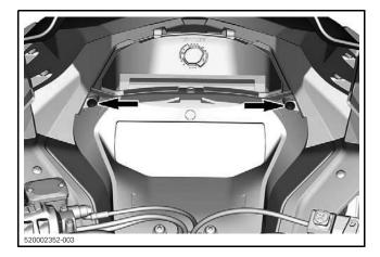
3. Remove the gauge retaining screws.
