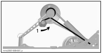
TYPICAL — RH SIDE 1. Adjust spring preload
