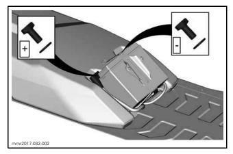
4. Remove battery hold down bracket.
