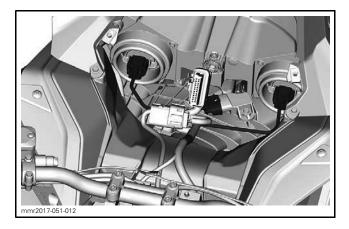
8. Loosen the air intake duct clamp.
