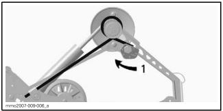
**TYPICAL** — LH SIDE 1. Adjust spring preload
