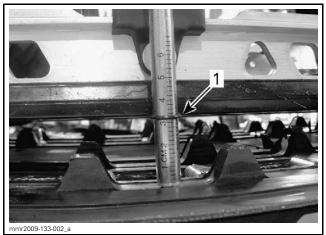
1. Deflection O-ring aligned with slider shoe
