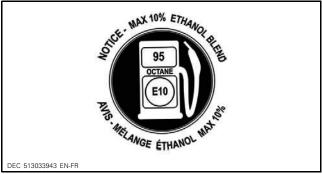
ON FUEL CAP - ON 600R E-TEC ENGINE (IN COUNTRIES USING RON OCTANE RATINGS)
