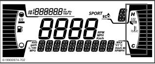
HEATED THROTTLE LEVER DISPLAY
