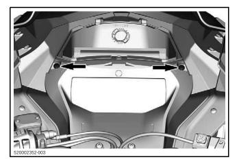
3. Remove the gauge support retaining screws.
