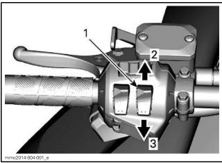
1. Heated throttle lever switch
