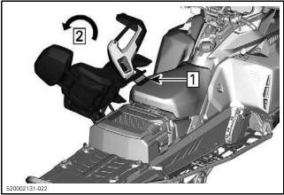
Step 1: Unlock seat latch Step 2: Tilt passenger seat
