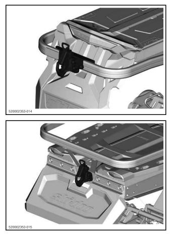
To open the hook, push and turn the handle to retract locking plate.
