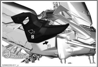
Step 1: Slide front Step 2: Pull out from side bottom pan
