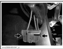
PUSH ON LOCKING TAB TO UNLOCK CONNECTOR
