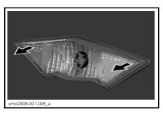
Turn and pull light socket to expose bulb.
