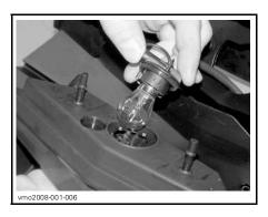
Push the bulb in and hold while turning counterclockwise to release.
