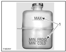
1. Level between marks when engine is cold
