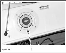
**TYPICAL — MAIN BATTERY CUT-OFF SWITCH** 1. Battery cut-off switch in OFF position
