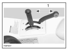
**TYPICAL — THROTTLE LEVER** 1. Must move freely
