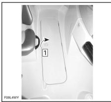
TYPICAL Step 1: Pull latch and lift cover
