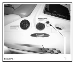
1. Flushing connector with its cap
