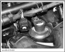
DISCONNECT IGNITION COIL CONNECTORS
