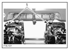
**TYPICAL** 1. Flushing connectors
