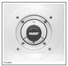
TYPICAL — MAIN BATTERY CUT-OFF SWITCH
