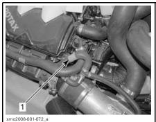
TYPICAL 1. Install hose pincher here
