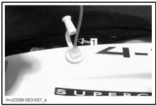
1. Can needle into lubrication fitting
