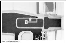
PASSENGER'S SIDE 1. Multi-purpose heating duct
