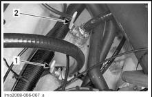
THRU-HULL VALVES — OPEN POSITION Starboard bag
