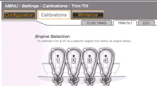
2) At the helm controls, lower the outboard to low trim position and touch the Set Calibration Point icon.
