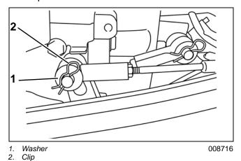
Tighten the control cable connector lock nut securely.
