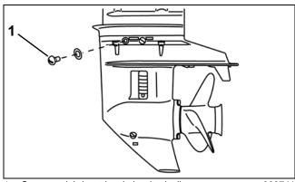
1. Gearcase lubricant level plug (typical)
