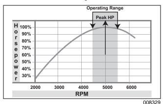
much pitch, the engine will operate below its normal range at full throttle. Power will be lost, and powerhead damage could occur. If the propeller blades have too little pitch, the engine will operate above its normal range and damage from overspeeding could occur.
