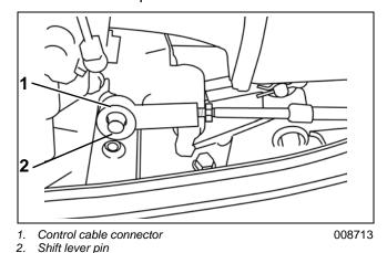
Secure the control cable connector with a washer and clip. Tighten the control cable connector lock nut securely.
