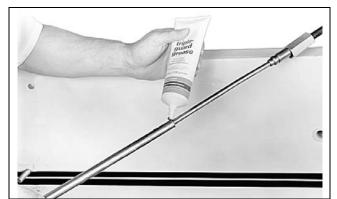
ABYC-approved mechanical steering cable.
