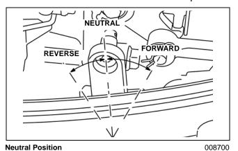
Turn the control cable connector to align with the shift lever pin. Install the control cable connector on the shift lever pin.
