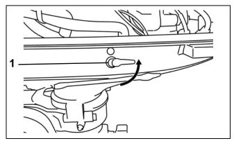
1. Fuel selector valve, remote fuel tank position
