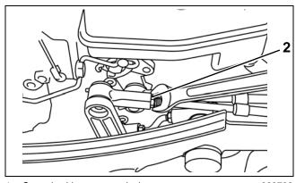
Control cable connector lock nut
