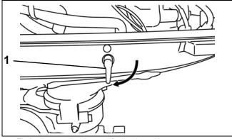
1. Fuel selector valve, integral fuel tank position
