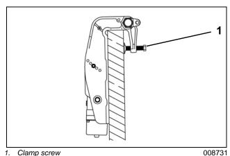
Bolt the engine to the boat's transom using the mounting hardware provided:
