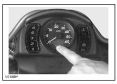
Press once to switch from odometer to tripmeter or vice versa. Press and hold to reset while in trip meter selection.
