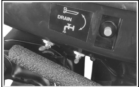
Tilt outboard to the full tilt position and turn so the drain valves are on the lowest side.
