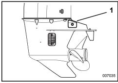
1. Anode anticorrosion
