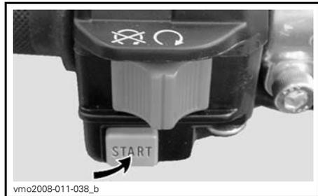
Release button immediately when engine has started.
