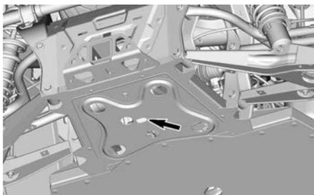
**ORIFICE D'ACCÈS AU BOUCHON DE VIDANGE.**
