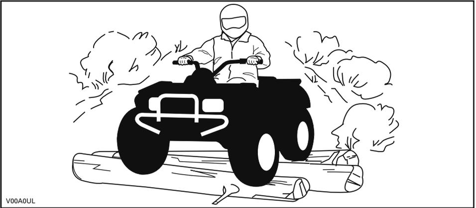
Even though there is an adequate suspension system on this vehicle there are “washboard” or rough terrain conditions that will make you feel uncomfortable and can even cause a back injury. “Posting” or riding in a crouched position will often be required. Slow down and allow your flexed legs to absorb part of the impact energy.
