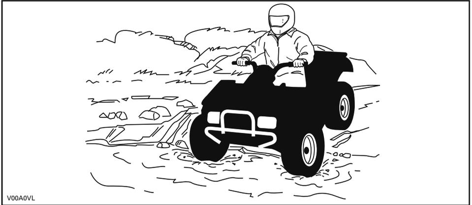
Water will affect the braking ability of your vehicle. Make sure you dry the brakes by applying them several times after the vehicle leaves the water. On 2-UP models, the vehicle braking distance may be affected when riding with a passenger. Safely reduce speed when riding with a passenger. Allow greater distance for braking.
