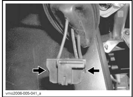
**PUSH ON LOCKING TAB TO UNLOCK CONNECTOR**
