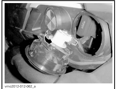
ROTATE BULB COUNTERCLOCKWISE
