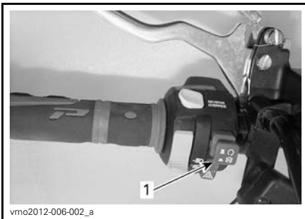
1. Emergency engine stop switch
