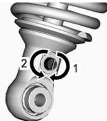
**DRUCKSTUFE STOßDÄMPFER - UNTEN AM**
