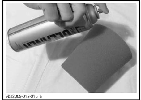
TYPICAL - SPRAY FOAM ELEMENT INSIDE AND OUT
