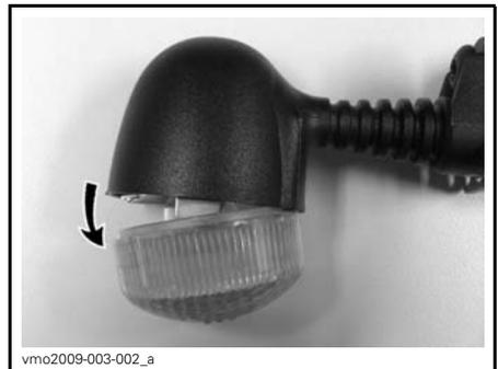
Push bulb in while turning it counterclockwise to release bulb from its socket.
