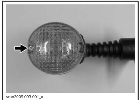
Tilt lens as shown to unlock it from housing.
