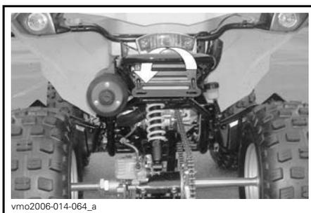
*EMPLACEMENT DES COURROIES DU PARE-CHOC ARRIÈRE*
