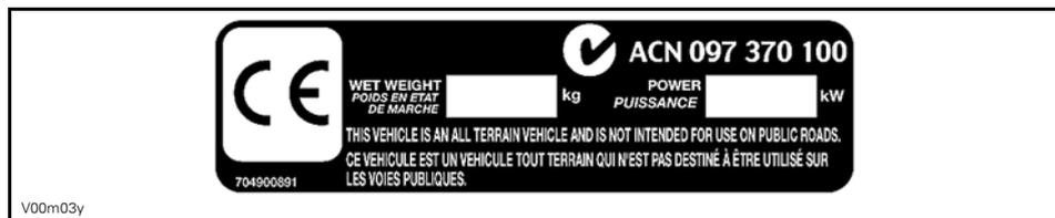
EMPLACEMENT: TUBE INFÉRIEUR AVANT DROIT DU CHÂSSIS
