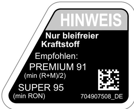
**1000R-MOTOREN - IN DER NÄHE DES KRAFTSTOFFTANKDECKELS**
