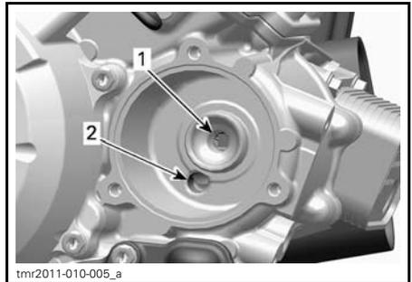
1. Outlet bore to the engine oil providing system
