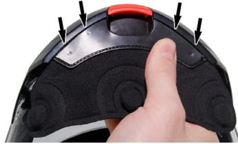
2. Press one by one on the plastic arrow snap to be sure each one is engaged in the chin plastic strip housing as shown.
