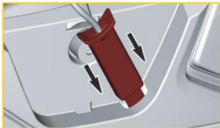
8. Pass the wire into the slot and hole.
