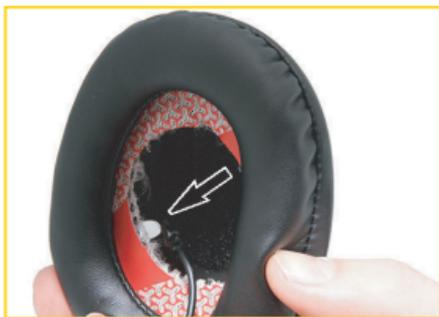
1.5. Using the Velcro, position and attach the speaker inside the NCS.
