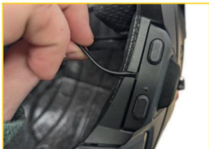
5. Slide the antenna into the hole and magnetically clip the user interface.
