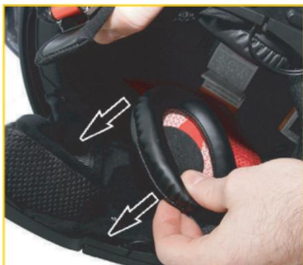
1.7. Reconnect the speaker cable with the BLACK female connector from the main unit. Repeat on the other side.
