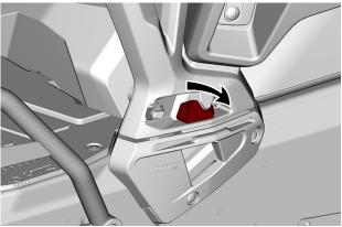
3. Pull the backrest upwards to remove..
