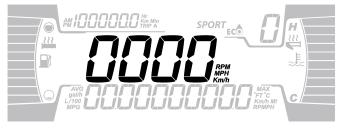
Display the RPM of the engine or the vehicle speed in Km/h or MPH.
