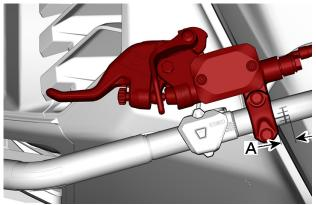
A. 0 to 9 mm (0 to 0.354 in) between the start of the handlebar mark and side of the brake lever
