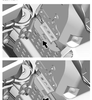
3. Insert belt guard tab between bottom pan and hook.
