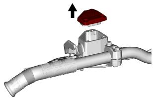
Add fluid as required. Do not overfill. Use only the recommended brake fluid.
