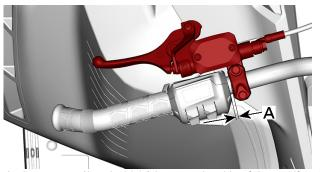
A. 0 to 15 mm (0 to 0.590 in) between the side of the multifunction switch and the side of the brake lever
