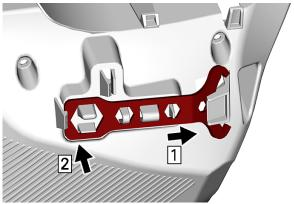
3. Slide the Pulley expander and headlight adjustment tool short end into hole.
