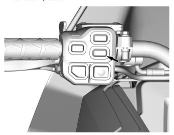
4. The desired set point appears on the display. To confirm, press the MENU (M) button or wait 5 seconds.
