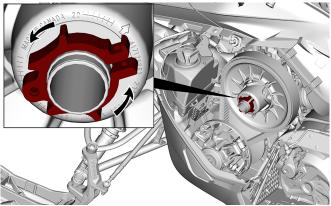
Screw the driven pulley expander in the threaded hole on the adjuster hub as shown.
