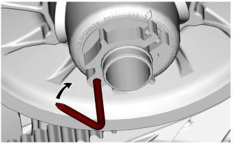
5. Open the driven pulley by screwing the tool in.
