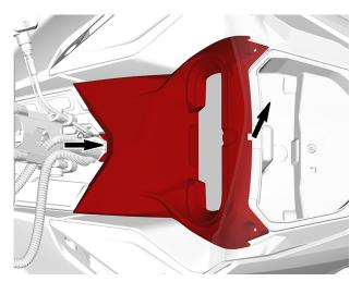
5. Disconnect the gauge connector and remove the support.
