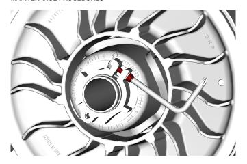
2. Using the suspension adjustment tool provided in the tool kit, turn the adjustment ring 1/4 turn at a time then rotate the driven pulley to properly set the belt between the pulley sheaves.
