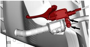
Locate the reference mark on the handlebar and respect the distance and rotation limits.
