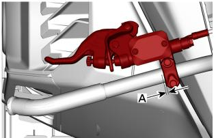
A. 0 to 5 mm (0 to 0.197 in) between the handlebar point and side of the brake lever
