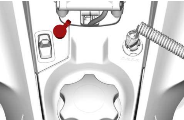
TYPICAL — DRIVER - ELECTRIC VISOR JACK CONNECTOR LOCATION
