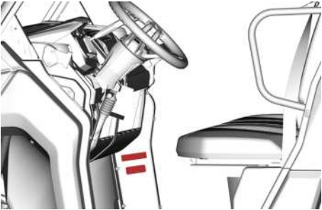
TYPICAL - VIN LABEL LOCATION
