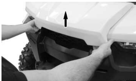
LIFTING FRONT SERVICE COVER EDGE.
