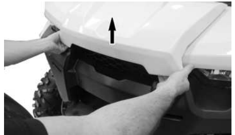
LIFTING FRONT SERVICE COVER EDGE.
