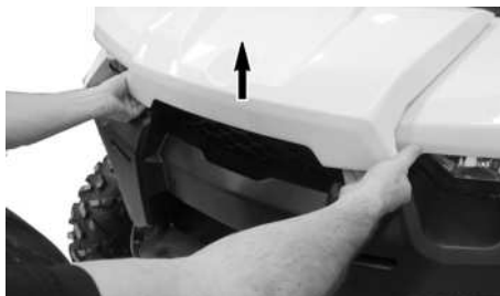
LIFTING FRONT SERVICE COVER EDGE.
