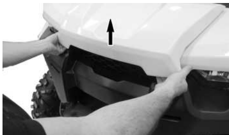
LIFTING FRONT SERVICE COVER EDGE.
