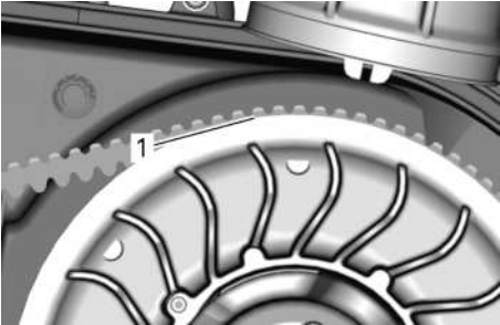
1. Lowest portion of cogs even with driven pulley edge
