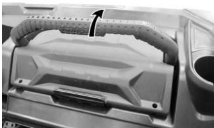
SECURING TOOL BOX IN PLACE
