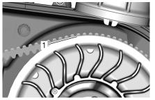
Lowest portion of cogs even with driven pulley edge
