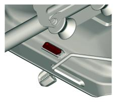
Pull up the rear of the cushion, then free the cushion from the seat frame by pulling it off towards the rear.
