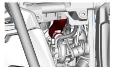
Open intercooler and crankcase hose support by removing the screw.
