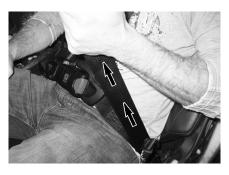
To loosen the seat belt, hold the lap belt with one hand and pull the red strap outwards.
