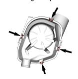
Remove the filter cartridge.
