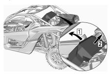
Remove CVT filter from vehicle.
