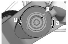
HIGH SPEED COMPRESSION DAMPING (USE A 17 MM WRENCH)
