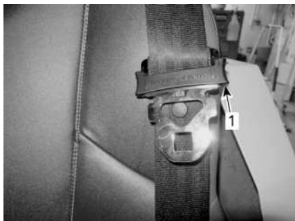
TYPICAL - LOCKED POSITION
