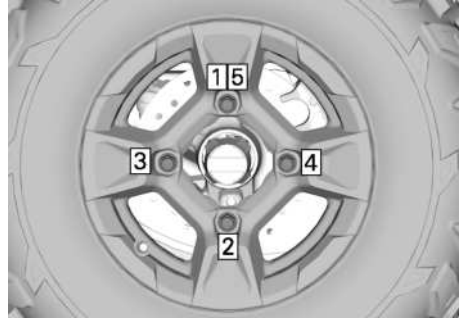
TIGHTENING SEQUENCE
