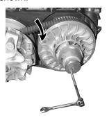
Installing the Drive Belt
