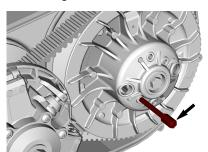
Turn the driven pulley until the lowest portion of the cogs on the external surface of the drive belt is even with the driven pulley edge.
