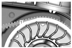
Lowest portion of cogs even with driven pulley edge
