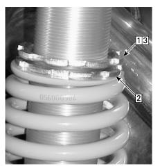
TYPICAL – SHOCK WITH THREADED ADJUSTMENT
