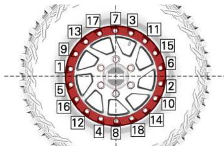
TYPICAL - TIGHTENING SEQUENCE
