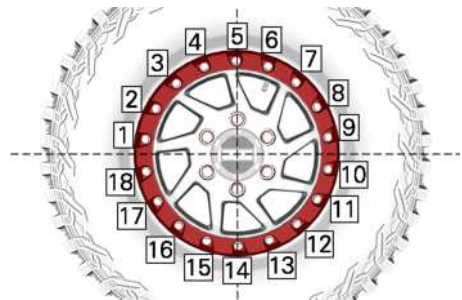
TYPICAL - FINAL TIGHTENING SEQUENCE
