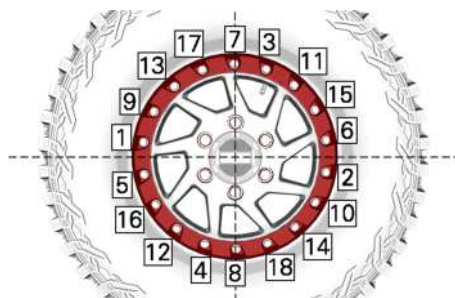
TYPICAL - TIGHTENING SEQUENCE
