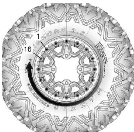
TYPICAL - FINAL TIGHTENING SEQUENCE
