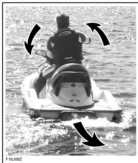
TYPICAL - STEERING DIRECTION REVERSED WHEN BACKING
