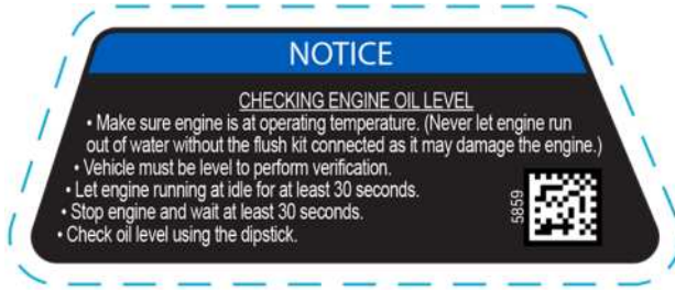
ENGINE OIL LEVEL - NOTICE LABEL
