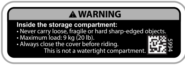
STORAGE COMPARTMENT - WARNING LABEL
